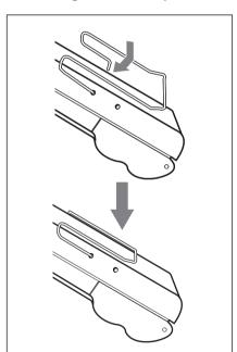
Insert one end of the belt clip into one of two holes on either side of the transmitter, and then insert the other end into the hole on the other side.
